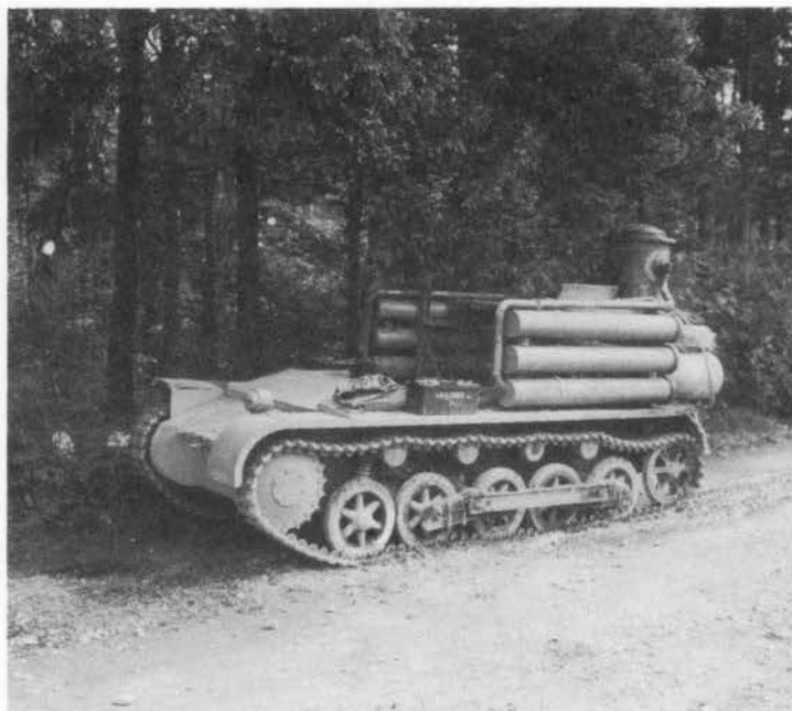
A charcoal-burning full-track armored vehicle near Salzberg, Austria, May 5, 1945
