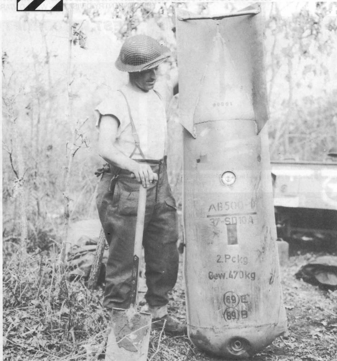
Photo shows a German anti-personnel bomb case of the type known as the "Butterfly" bomb. When the bomb is dropped, it falls a predetermined distance and the case is shot open, releasing a number of small delayed action bombs to fall in bivouac areas. They often lie for a day or two before exploding. Electrical connections, shown, activate the charge that opens the case. Anzio-Peter Beach Area, Italy, February 15, 1944.
